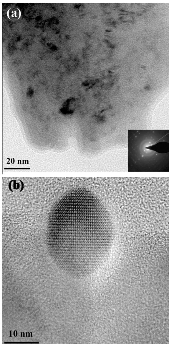
**Fig. 2.** TEM micrograph and SAD pattern of the stainless steel powder milled for 120 h (a). Related high-resolution TEM (b) where the atomic arrangement consideration indicates a crystalline zone embedded in the amorphous matrix.
