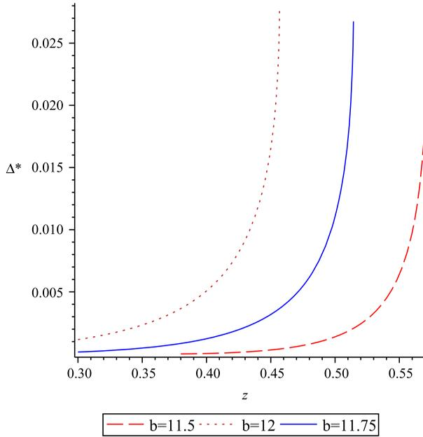
Figure 5. Case 2:  $\Delta^*$  versus  $z_\alpha$  for  $\mathcal{H} = 0.4722$ ,  $W_0 = 10$ ,  $R = 1.1$ ,  $\beta_0 = 0.045$ ,  $\vartheta = 10$ , for  $b = 11.5, 11.75, 12$ .
