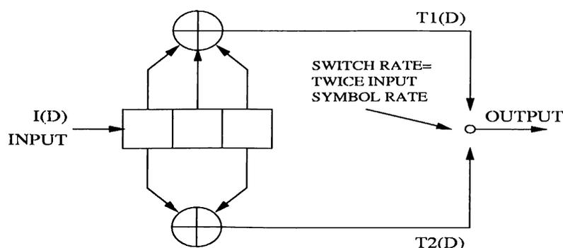
Figure 2.1: Encoder for a  $R = 1/2$ ,  $K = 3$  convolutional code
