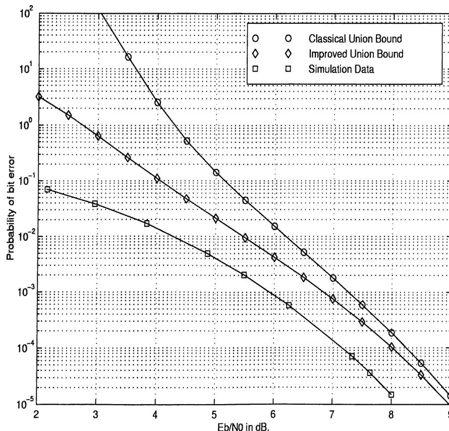
Figure 3.3: Probability of bit error for  $R = 1/2$ ,  $K = 3$  code over BSC with BPSK modulation
