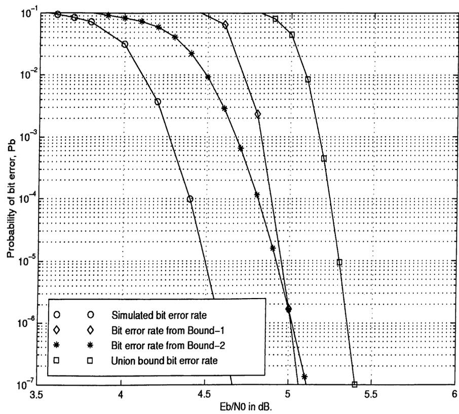
Figure 4.2: Bit error probability of ideally interleaved concatenated system over BSC with hard decision
