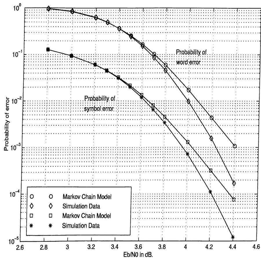
Figure 5.6: Word and symbol error probabilities for non-interleaved concatenated system over BSC and hard decision decoding
