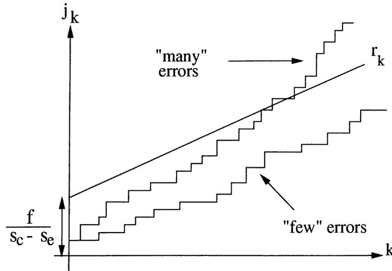
Figure 2.7: Barrier at  $r_k$  which separates paths with many and few errors
