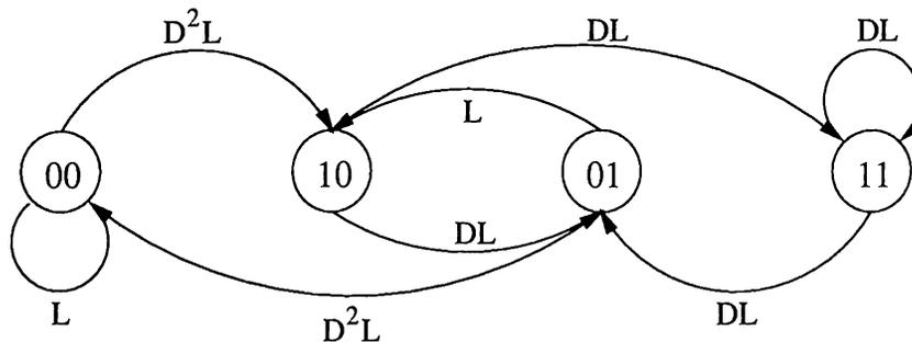
Figure 3.2: State diagram for rate-1/2 constraint-length-3 code
