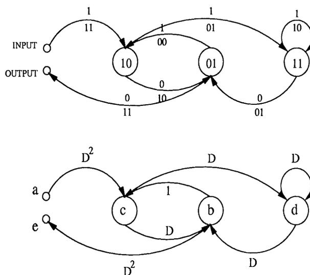
Figure 2.4: State and signal flow diagrams for the  $R = 1/2$ ,  $K = 3$  convolutional code
