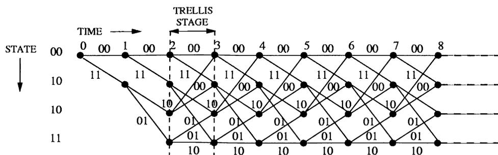
Figure 2.3: Trellis diagram for the  $R = 1/2$ ,  $K = 3$  convolutional code
