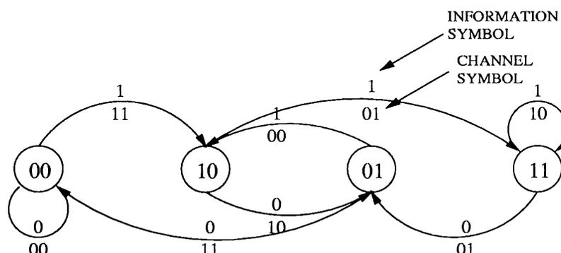
Figure 2.2: State diagram for the  $R = 1/2$ ,  $v = 2$  convolutional code
