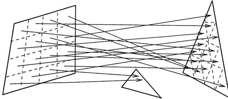
Figure 3.5: Rays fired from a quadrilateral to a triangle to detect occlusion.
