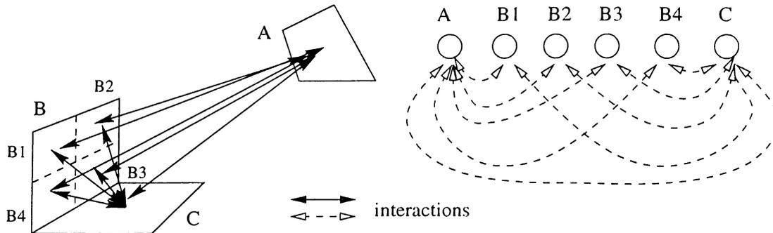
Figure 3.4: Sample interactions of progressive radiosity.
