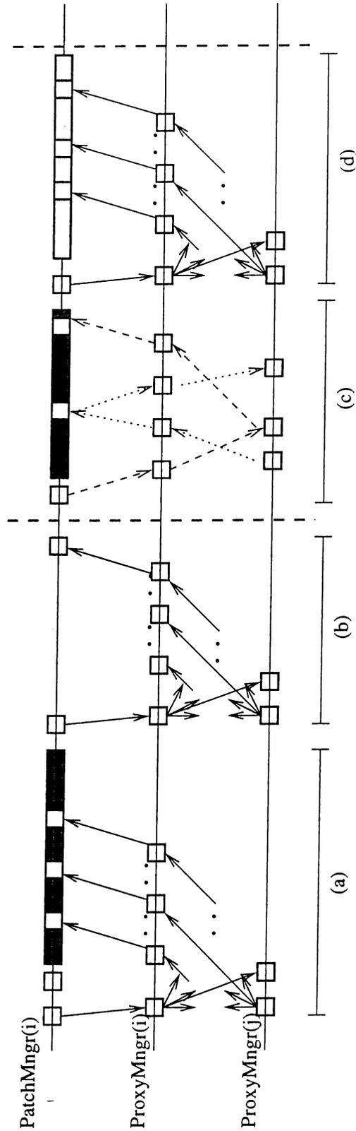
Figure 4.10: Work flow in an iteration (without migration).
