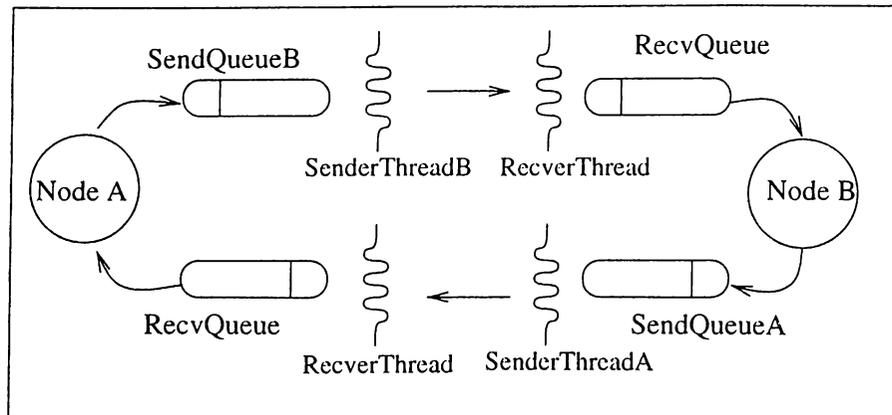
Figure 2.2: Communication model of  $N$ -sender 1-receiver version.
