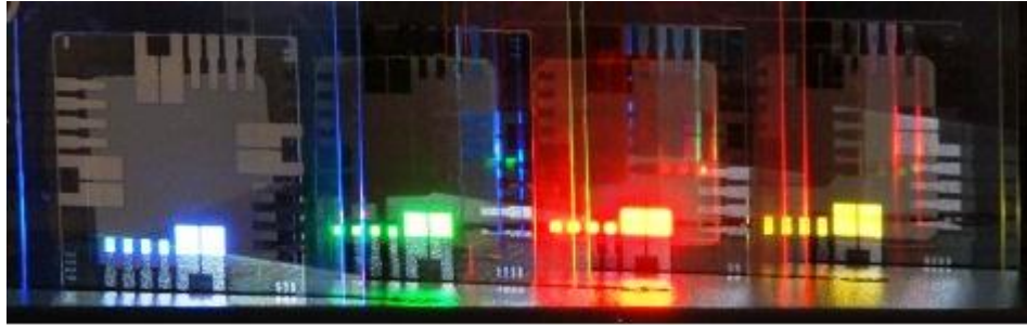
Figure 6.1. QD LEDs using electroluminescence process developed by QDVision.
