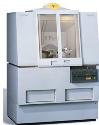
Figure 3.5. Panalytical X'pert Pro Multipurpose X-ray Diffractometer (MPD) located at UNAM.
