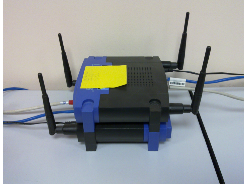
Figure 3.2: A BilMesh two-radio node (Mesh Access Point) consisting of two distinct APs.
