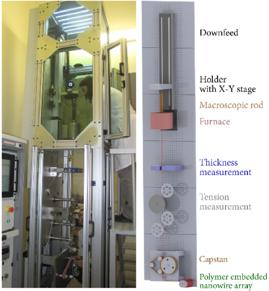
Figure 4.9: Computer controlled fiber tower facility and its schematic diagram
