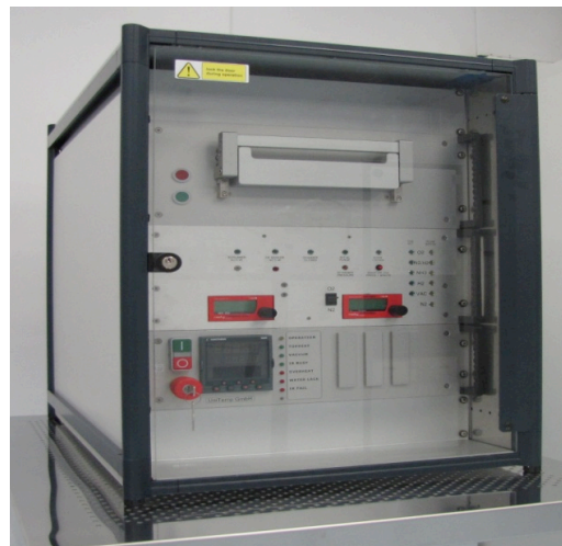
Figure 3.2: ATV-Unitherm (RTA SRO-704) rapid thermal annealing (RTA) system.
