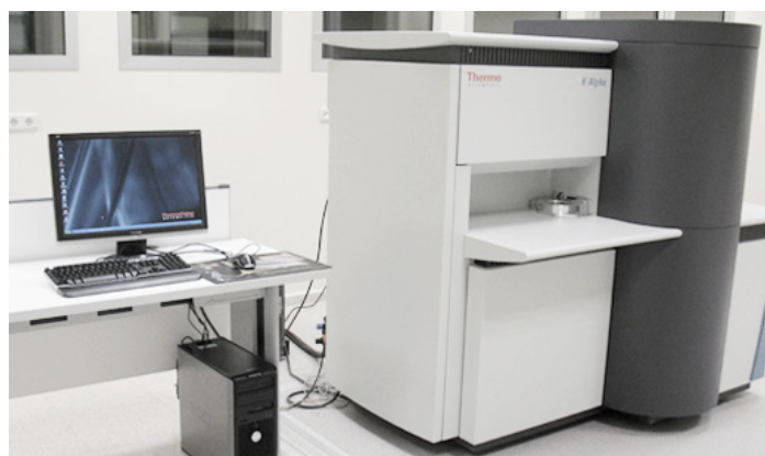
Figure 3.11: Thermo Scientific K-Alpha X-Ray photoelectron spectroscopy system.
