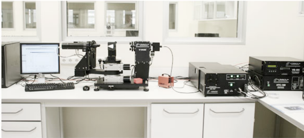
Figure 3.14: J.A. Woolam Co. V-VASE spectroscopic ellipsometer.
