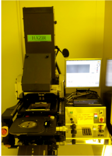
Figure 3.5: EVG 620 mask aligner used for the exposure of photoresist-coated wafers.
