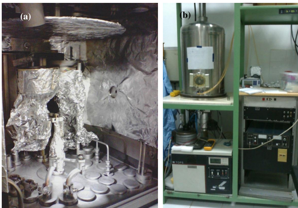
Figure 15. Photograph of (a) thermal and (b) e-beam (I) evaporation systems.
