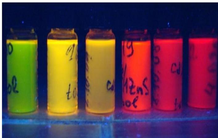
Figure 3.3.3 Our-synthesized CdSe core and CdSe/ZnS core/shell NQDs with different sizes emitting at correspondingly different wavelengths.
