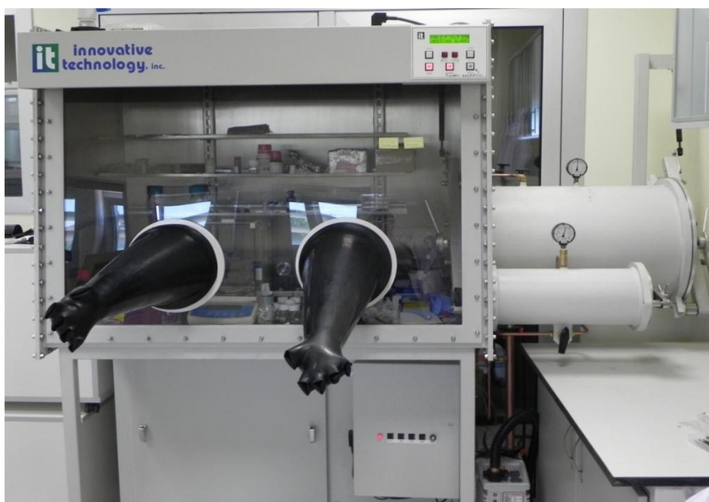
Figure 3.3.2 Glove box filled with nitrogen to create oxygen free environment for oxygen sensitive material processing.
