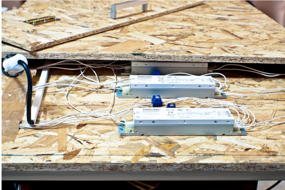
Figure 18 – Ultra Violet Exposure Unit Ballasts and Wiring
