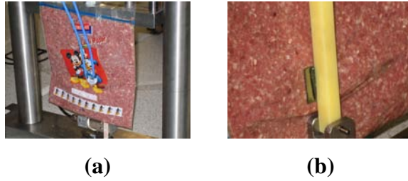
Figure 6.1.7. In vitro characterization with soft tissue (a) in front view showing antennas (b) in back view showing the sensor.
