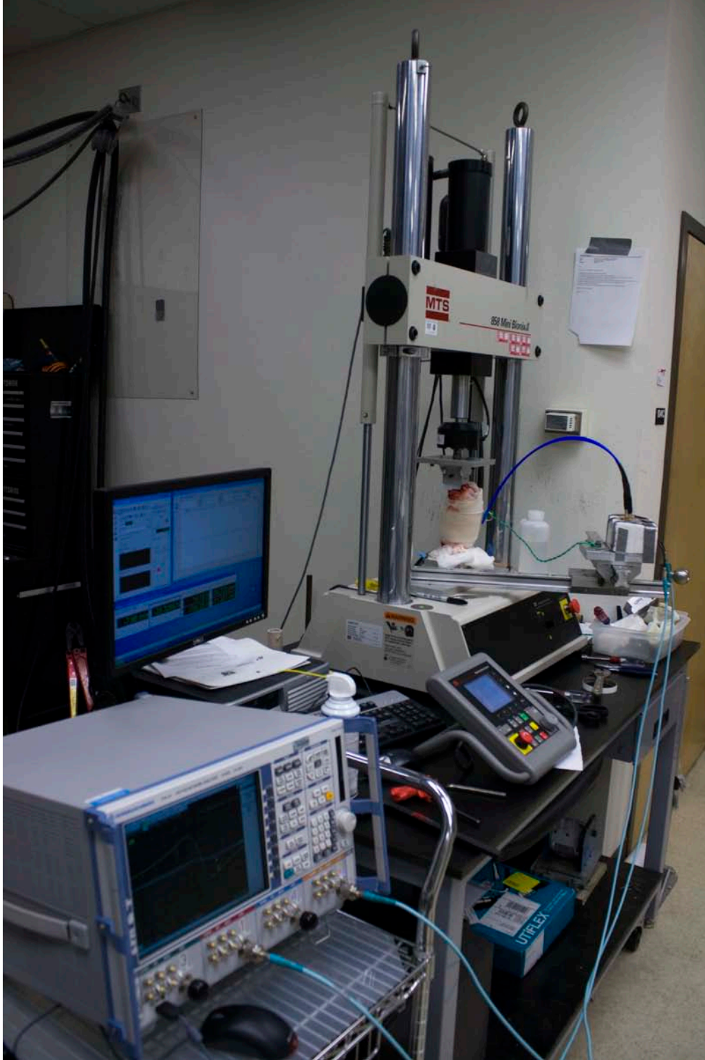
Figure 6.3.73. Experimental setup for sheep's femur experiments from different angles (a) – (h).
