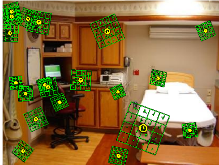
(a) A number of plotted SIFT descriptors on a hospital room image. The interest points are detected using Lowe's DoG detector.
