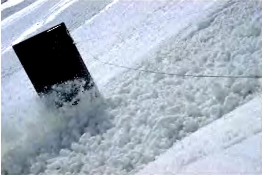
Figure 1.2: “Flowing avalanche impacting a wing-shaped structure in the Lauratet experimental site (France)” Balmforth et.al. [1]
