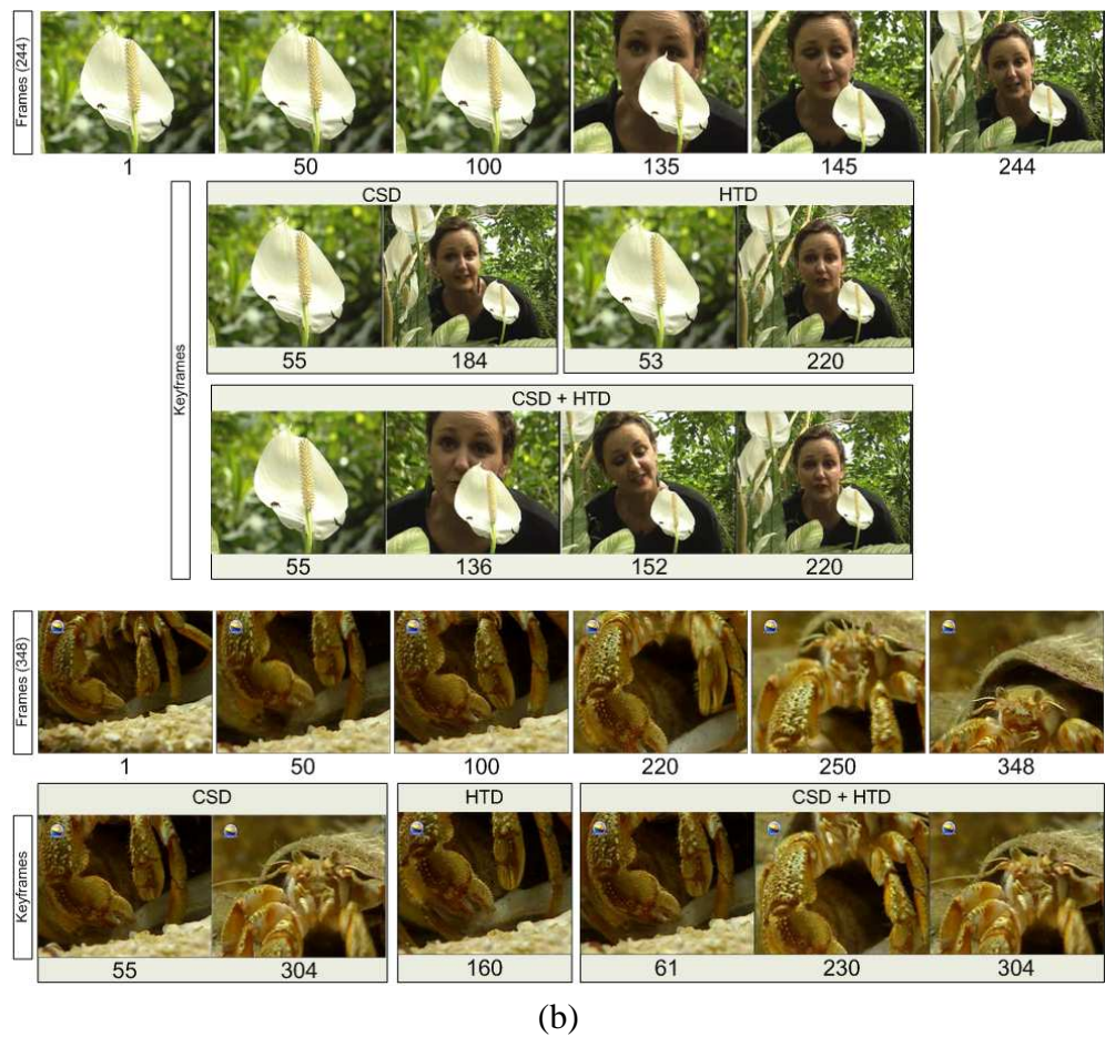
Figure 6.3: (a) Keyframe selection, (b) Keyframe examples. Frame numbers according to the start of the Shot are shown at the bottom of each image. CSD, HTD, CSD + HTD are the low-level descriptors used to select each group of Keyframes.
