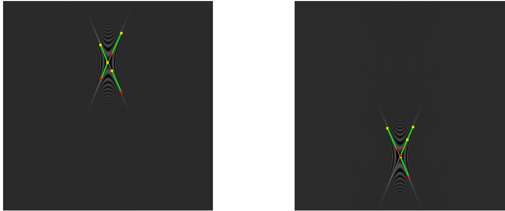
Figure 5.9: The lines detected by edge detection and Hough transform shown on Wigner transform output for column and row functions. All the figure properties are the same as Figures 5.6 and 5.7, respectively.
