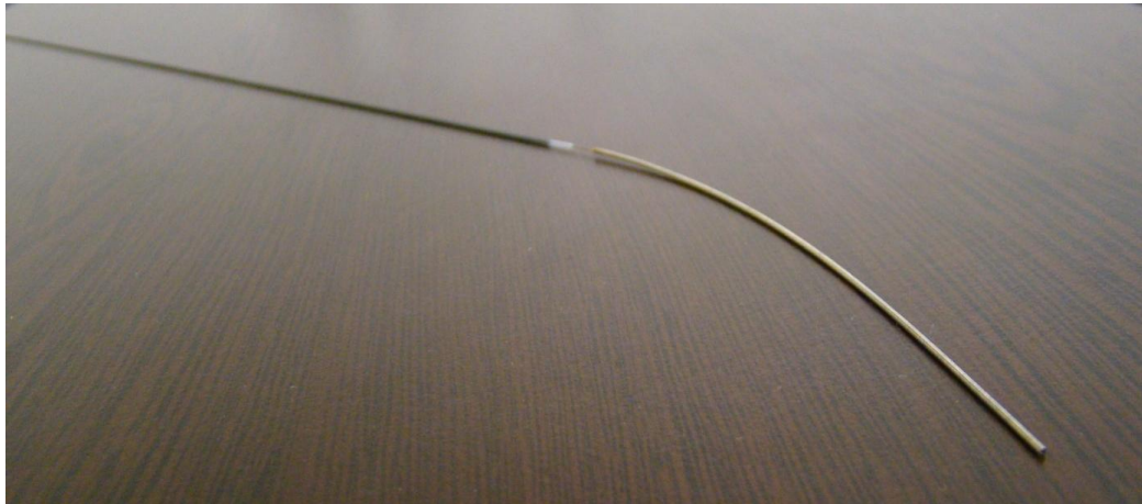
Figure 3.8: A picture of the assembled guidewire before being covered with heat shrink.
