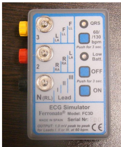
Figure 3.25: A picture of the ECG simulator which was used to test the functionality of the complete system
