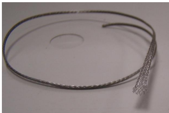
Figure 2.31: A picture of the copper braiding tube with 0.2 mm wall thickness that was used as an outer conductor of the coaxial portion.
