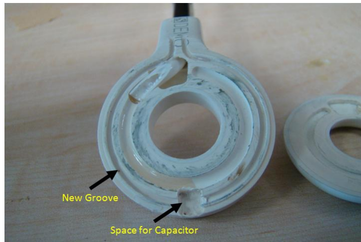
Figure 2.14: a picture of the modified Nucletron CT-MR ring applicator. A new groove of 1.5mm is opened for the loop coil and 4mm x 4mm x 4mm space is opened for the tuning capacitor.
