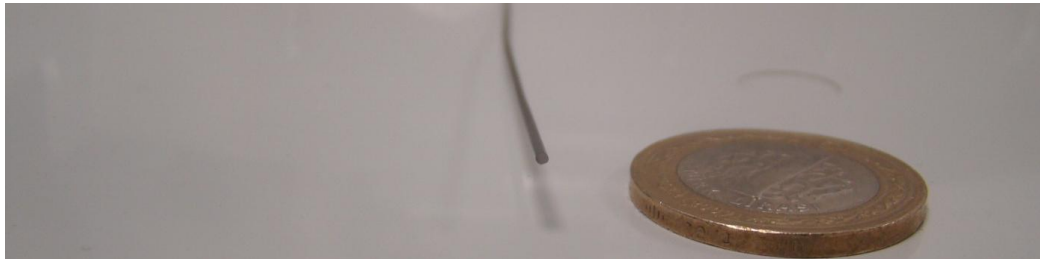
Figure 3.6: A picture of the polyester heat-shrink tubing with 0.96 mm outer diameter and 0.006 mm wall thickness.
