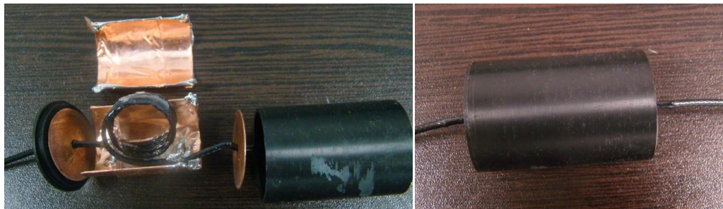
Figure 2.34: On the left hand side the internal structure of the explained balun is depicted. On the right side a side-view of the complete balun is given.
