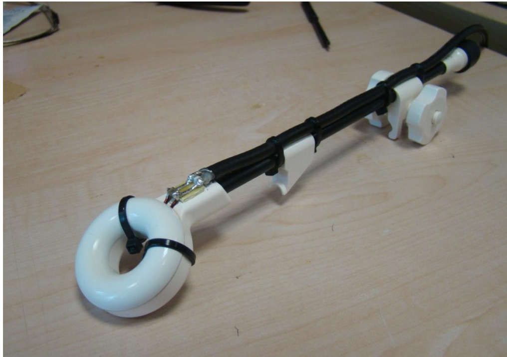
Figure 2.25: A picture of the final structure of the Nucletron CT/MR ring applicator with a loop coil placed inside.
