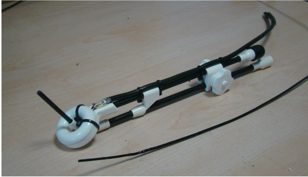
Figure 2.38: A picture of the two channel endocervix coil for HDRB
