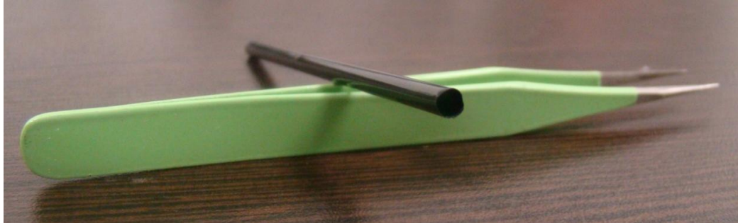
Figure 2.32: A picture of the polyester heatshrink tube with 3.35 mm outer diameter and 0.76 mm wall size before the expansion. This heatshrink was used as an outer isolator to provide electrical shielding and liquid isolation for the endocervical loopless probe.
