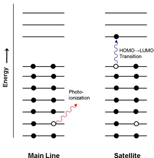
**Figure 3.25:** Illustration of the main line and a secondary excitation associated with HOMO→LUMO excitation
