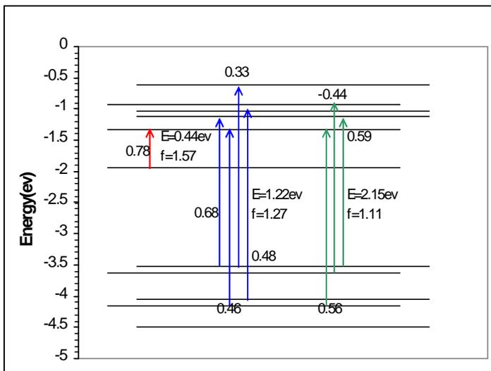
**Figure 3.10:** Orbital energies and excited state configurations for 12T<sup>-</sup>
