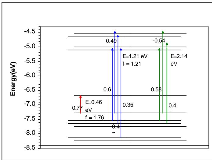
**Figure 3.11:** Orbital energies and excited state configurations for 12T<sup>+</sup>
