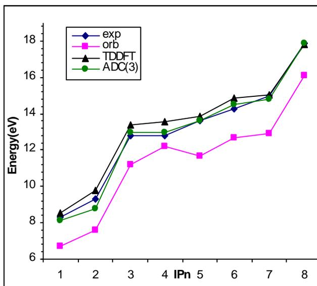
**Figure 3.16:** Comparison of SCF/TDDFT vertical excitations, DFT orbital eigenvalues and ADC(3) energy levels with experimental vertical IPs for pyrrole.
