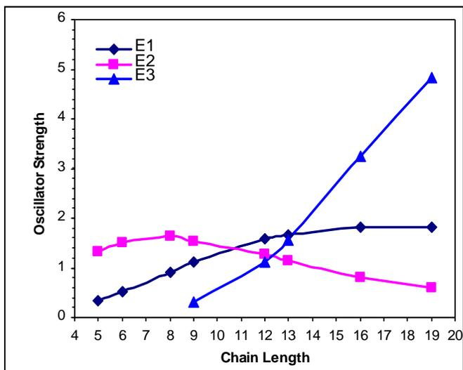
**Figure 3.8:** Oscillator strength vs. chain lengths of the three sub-band absorptions of 5T-19T anions
