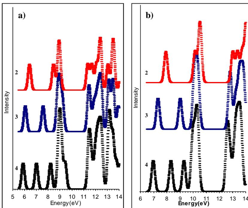
**Figure 3.22:** Theoretical UPS of furan (2-4) obtained by a) DFT $\epsilon_n$  and b) SCF/TDDFT.
