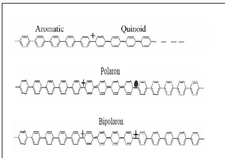
**Figure 1.3:** Formation of polaron and bipolaron defects in PPV
