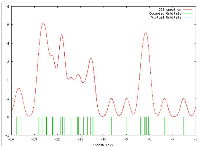
**Figure 1.5:** Theoretical modeling of the UPS. Discrete energy levels (bottom) are convoluted by 0.3 eV (FWHM).
