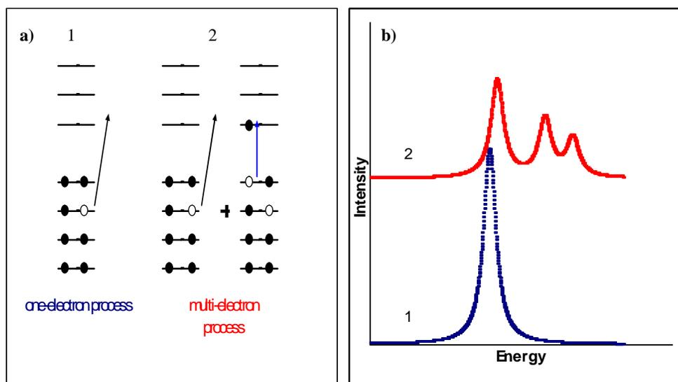
**Figure 1.6:** a) An illustration of one-electron and multi-electron photo-ionization b) appearance of the shake-up satellites in the spectra
