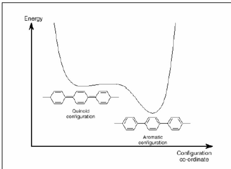
**Figure 1.2:** Potential energy diagram of aromatic and quinoid configurations of PPV.
