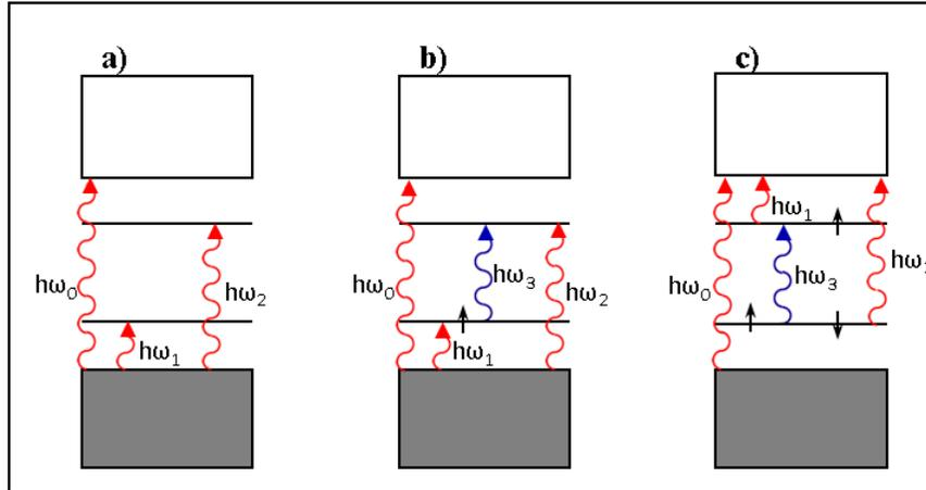
**Figure 1.4:** Optical excitations predicted for **a)** positively charged bipolaron and **b)** positively charged polaron. Note that there is an additional transition due to occupancy of lower level at mid-gap
