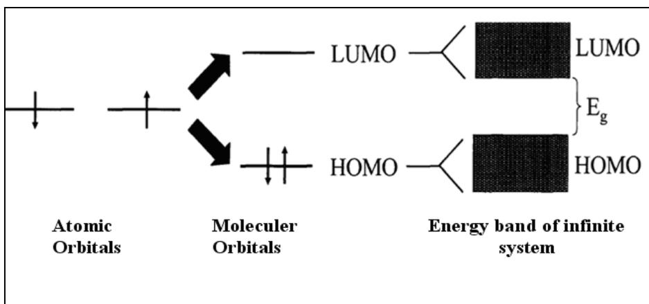
**Figure 1.1:** Formation of band structure from molecular orbitals in a qualitative picture
