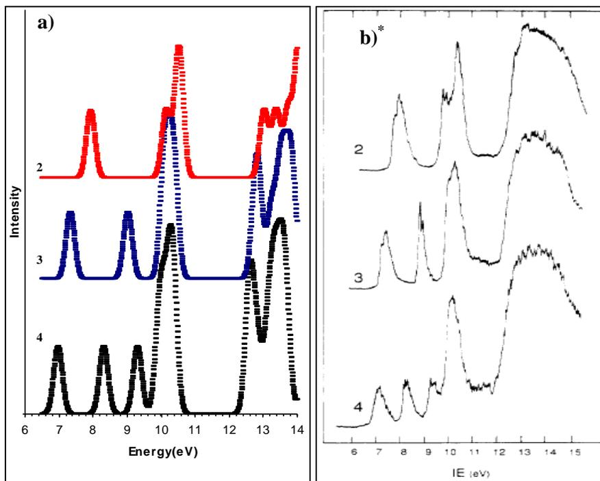
**Figure 3.19:** a) Theoretical and b) experimental UPS of oligofurans (2-4)
