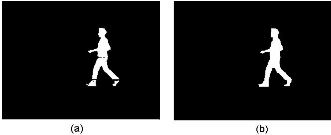
Figure 3.2: a)Object silhouette obtained from background subtraction b)Object silhouette after image enhancement operations
