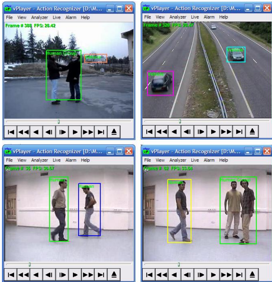
Figure 3.8: Sample screenshots from real-time object tracking and classification system.
