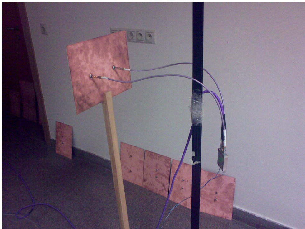
Figure 5.10: The 2 element receiver array with the switch and cable attached.
