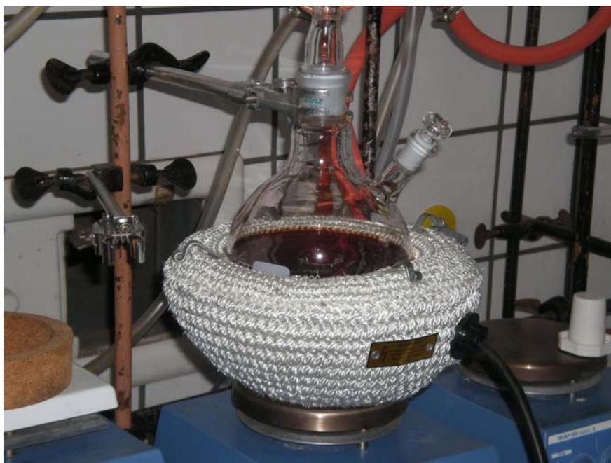
Figure 2.3.2 Red-brown mixture after the formation of CdTe nanocrystals (with our Phoremost collaborators).
