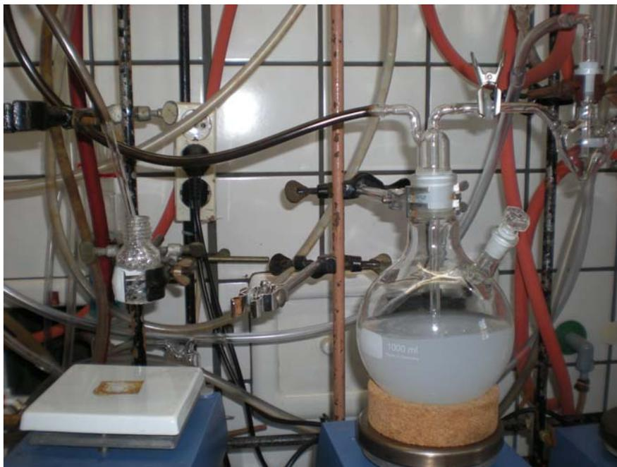
Figure 2.3.1 Apparatus of water-soluble CdTe semiconductor nanocrystals synthesis. After the regulation of pH to 11.8-12.0 solution becomes slightly turbid and clear (with our Phoremest collaborators).
