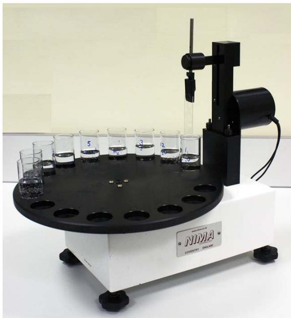
Figure 3.2.1 Multi-vessel dip coater (Nima Technology) at Demir Lab at Bilkent.
