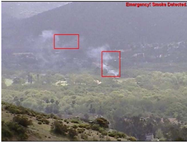
Fig. 5 A snapshot from an independent test of the system by the Regional Technology Clearing House of San Diego State University in California in April 2009. The system successfully detected the test fire and did not produce any false alarms. The detected smoke regions are marked with bounding rectangles.
