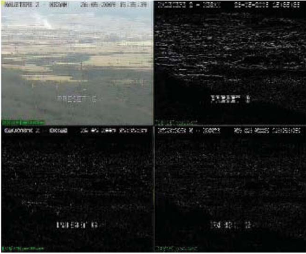
Fig. 4 Single-level wavelet decomposition of the snapshot image in Fig. 3 obtained using h_{lp}[n] = \{\frac{1}{4}, \frac{1}{2}, \frac{1}{4}\} and h_{hp}[n] = \{-\frac{1}{4}, \frac{1}{2}, -\frac{1}{4}\} as low and high-pass filters, respectively.
