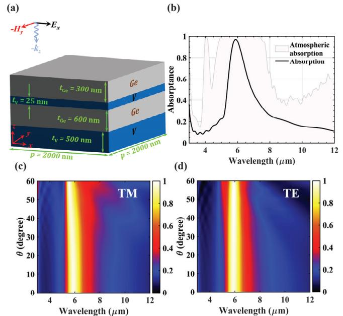
Fig. 1. (a) Schematic diagram of the proposed multilayer absorber. (b) The simulated absorbance of the proposed structure versus wavelength. The atmospheric absorption band [shown as the light area] is modeled by the US standard atmosphere compositions at the vertical distance of 5 km [12]. Numerically calculated the dependence of the absorption performance of the structure on the incident angle for (c) TM and (d) TE polarizations.
