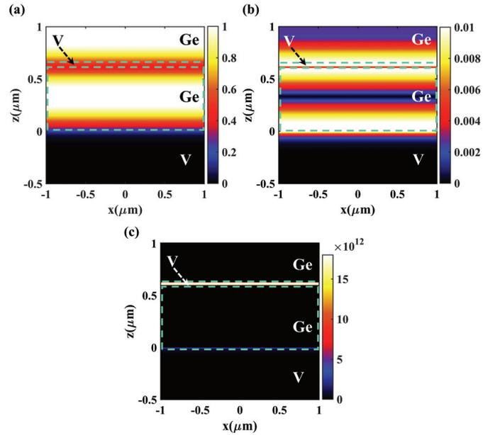
Fig. 2. Absolute values of the total electric- (a) and magnetic-field (b) distributions of the proposed structure at the resonance wavelength of 5870 nm. (c) Absolute value of the absorbed-power density at the same resonance wavelength.
