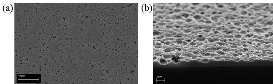
**Figure 9.** a) SEM image of photochemically etched Si surface. b) 50 nm Ag deposited rough Si surface that is the SERS substrate.
