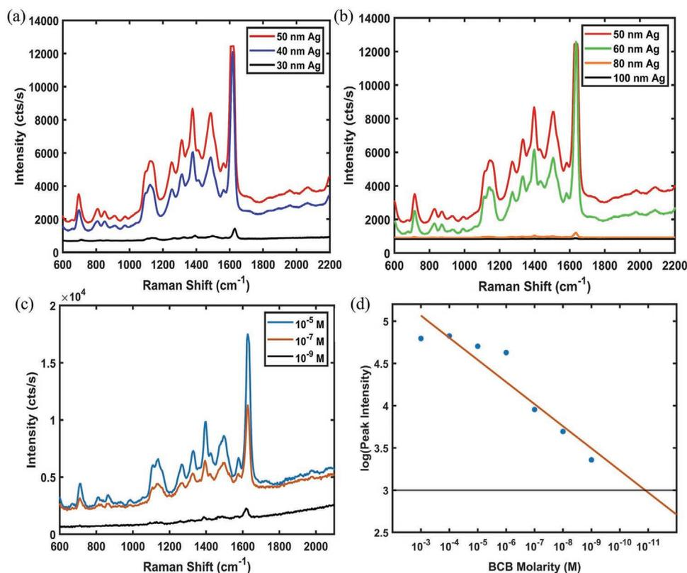
**Figure 2.** a) Ag deposition thickness impact on SERS signal varying from 30 up to 50 nm. b) Ag deposition thickness impact on SERS signal up to 100 nm. c) Raman spectra obtained at different BCB concentrations adsorbed on 50 nm Ag deposited substrates under 532 nm excitation. d) Determination of LoD from  $\log(\text{Raman signal})$  versus  $\log(\text{concentration})$  curve with a linear fit, horizontal line indicates the lowest discernible signal intensity of the Raman spectra.
