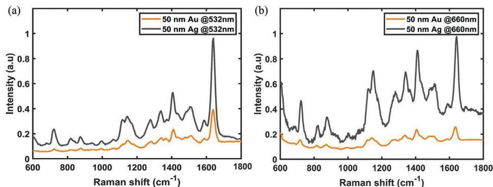
**Figure 3.** SERS spectra of both 50 nm deposited and  $10^{-5}$  M BCB adsorbed Ag and Au substrates under a) 532 nm and b) 660 nm laser excitation.
