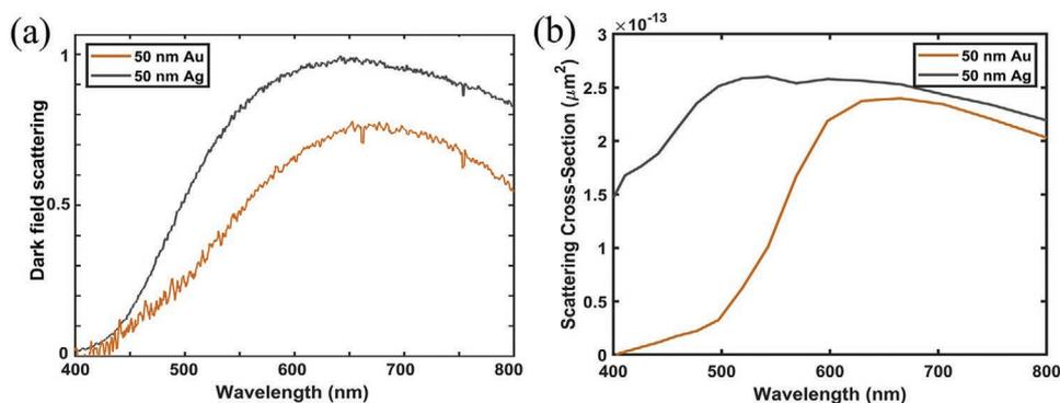
**Figure 6.** a) Normalized scattering spectra of the 50 nm deposited Au and Ag substrates on Si nanoholes obtained via dark field scattering. b) Scattering cross-sections calculated using FDTD simulations.
