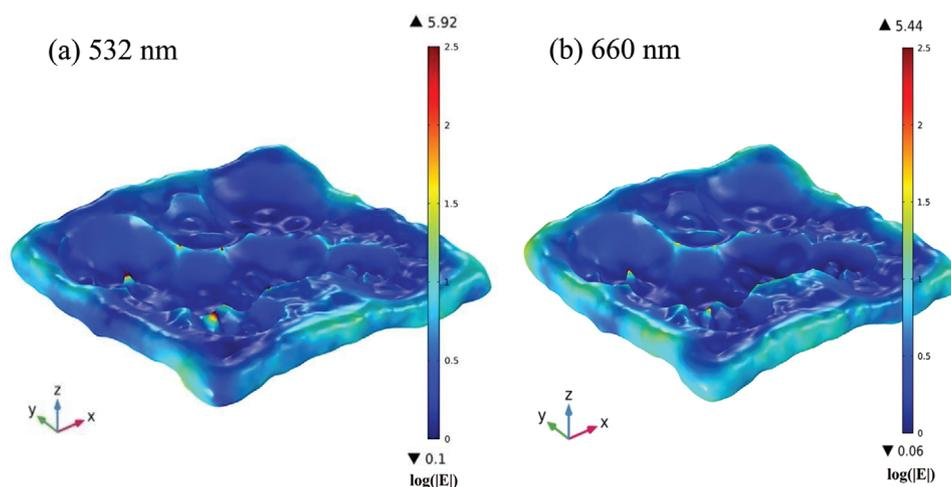
**Figure 7.** FEM simulation of the nanostructured 50 nm Ag substrate surface under both a) 532 and b) 660 nm illumination as used in SERS experiments using COMSOL. Color bars denote the electric field strength in logarithmic scale.
