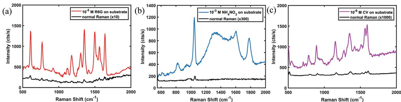
**Figure 8.** Raman spectra of a)  $10^{-5}$  M R6G dye molecule, b)  $10^{-3}$  M  $\text{NH}_4\text{NO}_3$ , and c)  $10^{-6}$  M CV dye molecule under 532 nm excitation using substrates with the same structuring parameters and 50 nm Ag compared with their normal Raman spectra.
