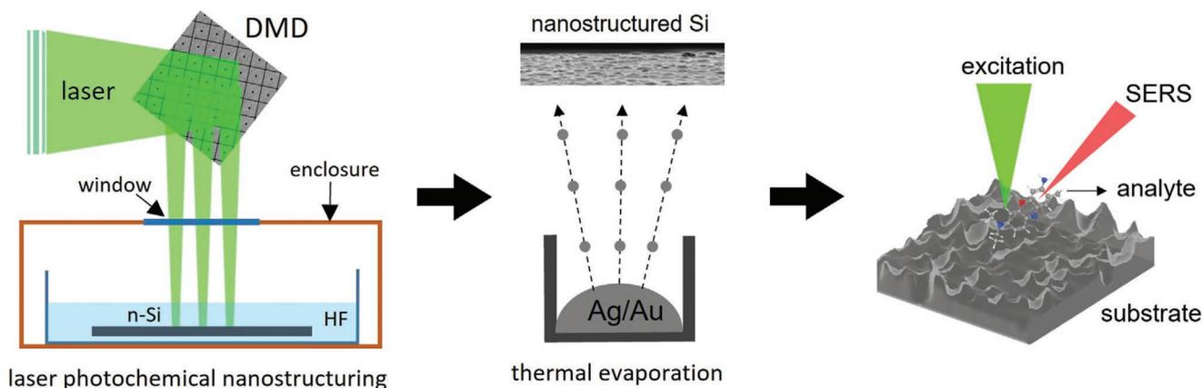
**Figure 1.** Two-step fabrication of novel SERS substrates from left to right: laser photochemical nanostructuring of Si surface followed by thermal evaporation of Ag/Au and assessment of its SERS potential using a Raman reporter molecule.
