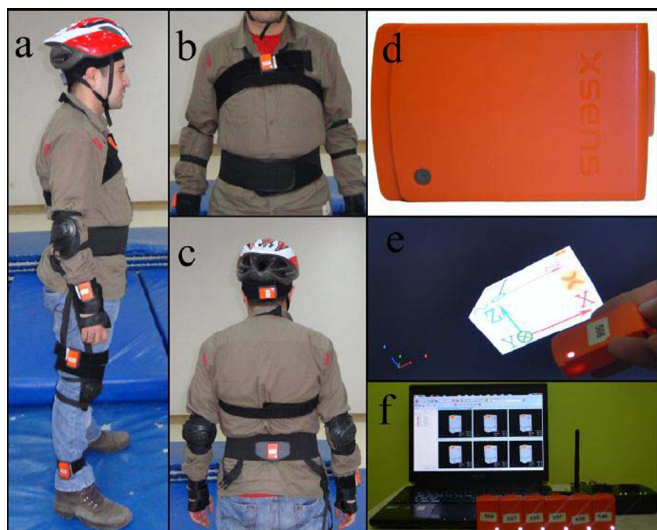
Fig. 3. a)-c) Configuration of the sensor units on the subject's body, d) MTw sensor unit, e) axes of a sensor unit, f) connection to a PC and the interface [12].
