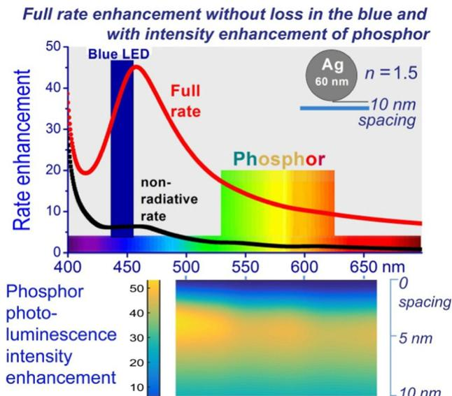
**Fig. 7** A brief summary of the LED performance enhancement by metal nanoparticles (silver, 60 nm diameter). The full rate can be enhanced both for electroluminescence in the blue (LED range) and for photoluminescence in the phosphor range whereas the non-radiative decay does not change dramatically. At the same time, phosphor emission intensity can be enhanced as well depending on metal-phosphor spacing (shown in the bottom)
