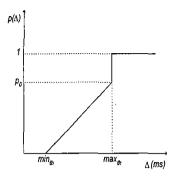
Fig. 2. The traffic splitting function  $p(\Delta)$
