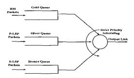
Fig. 1. Queuing architecture for MPLS switches
