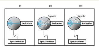
**Fig. 5** Illustration of the quantum efficiency measurement methodology: (i) the measurement of the excitation spectrum without sample, (ii) the measurement of the spectrum when the sample is directly excited by the light source, and (iii) the measurement of the spectrum when the sample is excited by the light that scatters from the surface of the integrating sphere.
