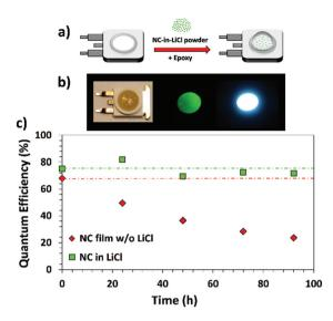
**Fig. 4** (a) Schematic image of NC-in-LiCl film preparation onto LED for the temperature stability test. (b) Real colour images of the NCs-in-LiCl on a blue LED under ambient lighting, UV illumination at 366 nm, and when LED is driven, from left to right. (c) Quantum efficiency variation of the NCs with and without LiCl encapsulation as a function of time when they are integrated on the blue LED driven at a high current level for 96 h (four days).
