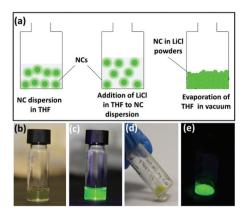
**Fig. 1** (a) Schematics of NC encapsulation into LiCl salt. The real colour images of NC dispersion in THF (b) under ambient lighting and (c) UV illumination at 366 nm. The real colour images of the NCs-in-LiCl powders (d) under ambient lighting and (e) UV illumination at 366 nm.
