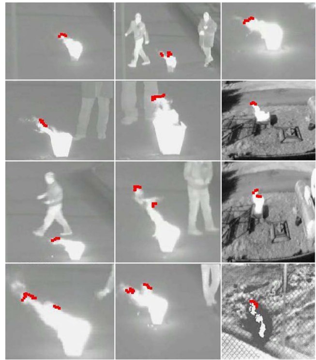
Fig. 9 Image frames from some of the test clips with fire. Pixels on the flame boundaries are successfully detected.
