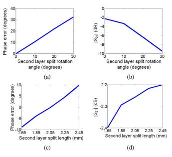
Fig. 4. The phase and magnitude characteristics with respect to the changes in the split parameters in one layer at 8.8 GHz. (a) Phase error and (b) the transmission magnitude of  $s_{21}^{rl}$  when the angular position of the split in the second layer changes with respect to the split in the first layer. (c) Phase error and (d) the transmission magnitude of  $s_{21}^{rl}$  with respect to the change in the length of the split in the second layer.
