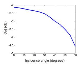
Fig. 3. Magnitude of  $s_{21}^{rl}$  with respect to the incidence angle at 8.8 GHz.
