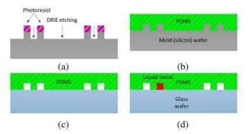
Fig. 5. Fabrication process flow: (a) mold wafer preparation via DRIE process, (b) PDMS coating, curing, and peeling off, (c) PDMS-to-glass bonding process, and (d) Liquid metal injection.
