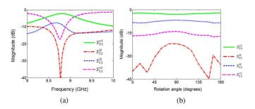
Fig. 2. Magnitude of the scattered waves with respect to (a) frequency and (b) rotation angle at 8.8 GHz.
