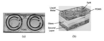
Fig. 7. (a) One layer of the fabricated double layer transmitarray unit cells for the rotation angle of  $20^{\circ}$ . (b) The double layer transmitarray unit cell with dimensions 22.86 mm  $\times$  10.16 mm  $\times$  9 mm.
