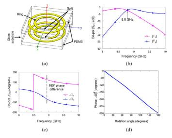
Fig. 1. (a) Geometry of the double layer nested ring-split ring transmitarray unit cell. Simulated (b) magnitude and (c) phase of the co-pol transmission coefficients for x- and y-polarized incident waves. (d) The transmission phase, the phase of  $s_{21}^{x1}$ , with respect to the rotation angle at 8.8 GHz.
