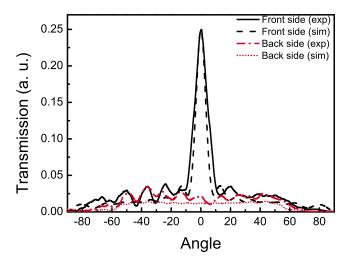
FIG. 4. (Color online) Experimental and simulated angular distributions of transmission at f=9.8 GHz for sample A at  $\theta$ =30°. Positive angles represent the right-hand side of the structure, while negative angles represent the left-hand side of the structure.
