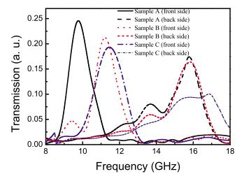
FIG. 2. (Color online) Calculated transmission for samples A–C at  $\theta$ =30°. Illumination side is specified in brackets.
