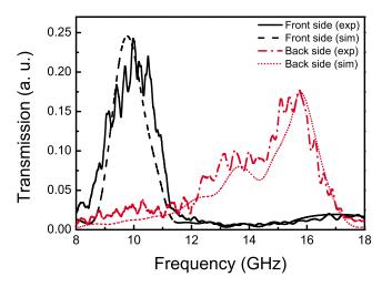
FIG. 3. (Color online) Experimental and simulated transmission results for sample A at  $\theta$ =30°.
