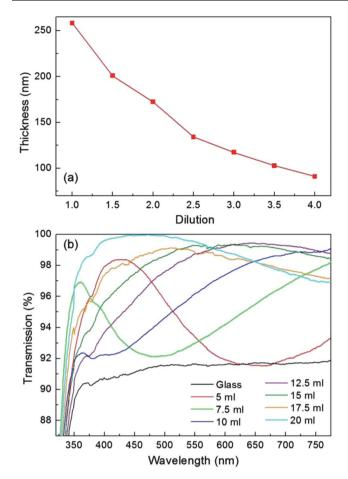
**Fig. 8** (a) Effect of dilution of the suspension on the thickness of T60 film, indicating that the thickness can be controlled by dilution in the range of 260–90 nm. (b) The transmission of T60 film for different thicknesses. As the film gets thinner, the transmission maximum shifts to lower wavelengths.
