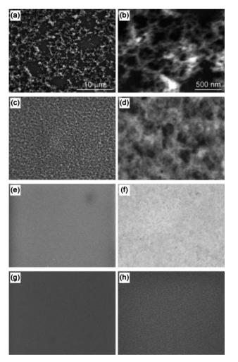
Fig. 1 SEM micrographs of (a,b) T0, (c,d) T25, (e,f) T60 and (g,h) T80 films, which indicate that the surface coverage and uniformity of the ormosil films improve with increasing amount of TEOS, in addition to decreasing pore sizes.
