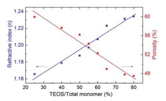
**Fig. 5** Effect of the TEOS fraction on the refractive index and percent porosity. As the TEOS fraction increases, the refractive index increases due to decreasing porosity. This dependence of refractive index on the TEOS fraction enables the preparation of thin films with different refractive indexes which can be used with different substrates.
