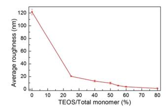
**Fig. 4** Average surface roughness as a function of the TEOS fraction graph, indicating that as the TEOS ratio increases, the average surface roughness decreases. Even 25% TEOS addition causes around a 100 nm decrease in the average roughness.
