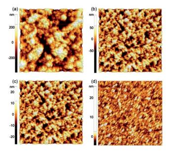
Fig. 3 AFM images of (a) T0, (b) T25, (c) T60 and (d) T80 films taken from a  $10 \times 10 \ \mu\text{m}^2$  area, showing that as the TEOS fraction increases, the average roughness and cluster size decrease.
