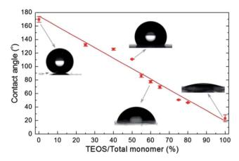
**Fig. 10** Change of contact angle with respect to the TEOS fraction, showing that as the TEOS fraction increases the surface becomes more hydrophilic. Inset: photographs of T0, T40, T60 and T100 films are used to visualise how water droplets spread on each surface, respectively.
