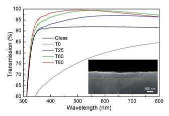
**Fig. 6** Transmission spectra of double side coated substrates with T0, T25, T60 and T80 films and a bare glass slide. The MTMS-TEOS hybrid films exhibit AR properties on the glass substrate with the transmission reaching 99.5%. The inset shows a cross sectional SEM image of the T60 film, indicating the homogeneity in thickness.
