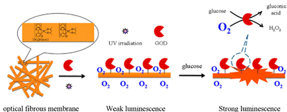
Fig. 13 Schematic illustration of the GOD/EOF quickly detecting glucose [Reprinted with permission from [218] © 2013, American Chemical Society]
