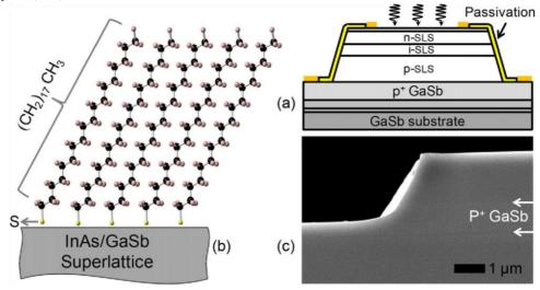
**Figure 1.** (a) Schematic side view of the InAs/GaSb superlattice p-i-n photodiode structure. (b) Schematic of ODT on the superlattice surface. (c) SEM micrograph of a SAM of ODT-passivated type-II InAs/GaSb photodiode.
