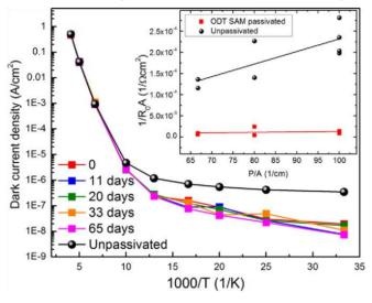
**Figure 4.** Temperature-dependent dark current density for the unpassivated and ODT SAM-passivated type-II InAs/GaSb superlattice  $400 \times 400 \mu m$  photodiodes at -0.1V bias voltage. Inset shows the dependence of dynamic resistance—area product at zero bias versus perimeter-to-area ratio for the unpassivated and passivated devices at 77K.
